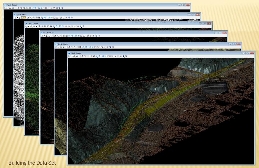
Photo Draping added to DTM Triangles
