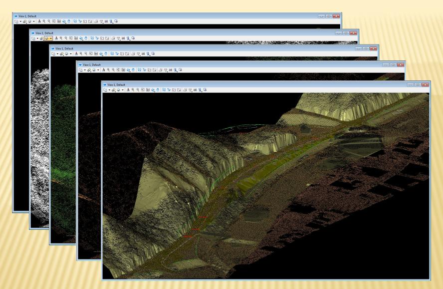
Building the Data Set Ground DTM rendered from Aerial LiDAR
