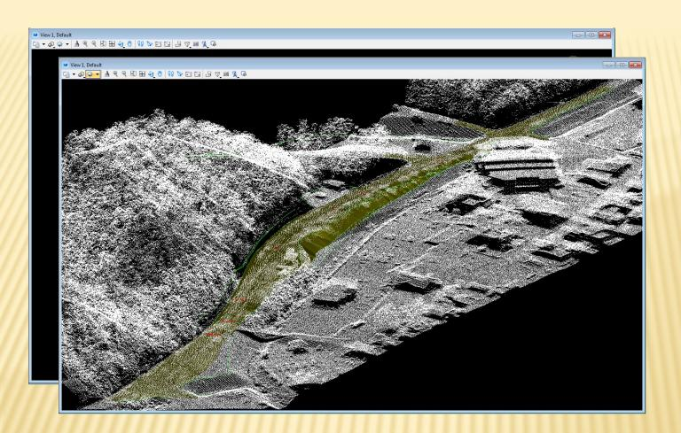
Building the Data Set Aerial LiDAR added for ground base
